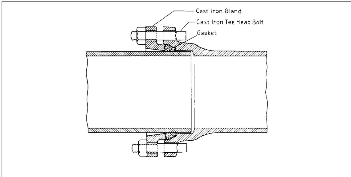
Fig. 19. Standardized mechanical joint.
