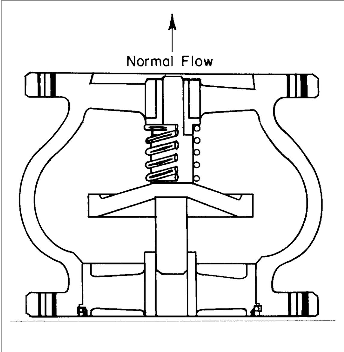
Fig. 7. Anti-water hammer check valve.
