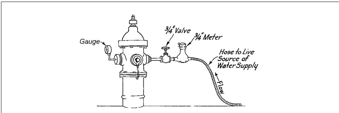
Fig. 43. Metering method of leak detection.
