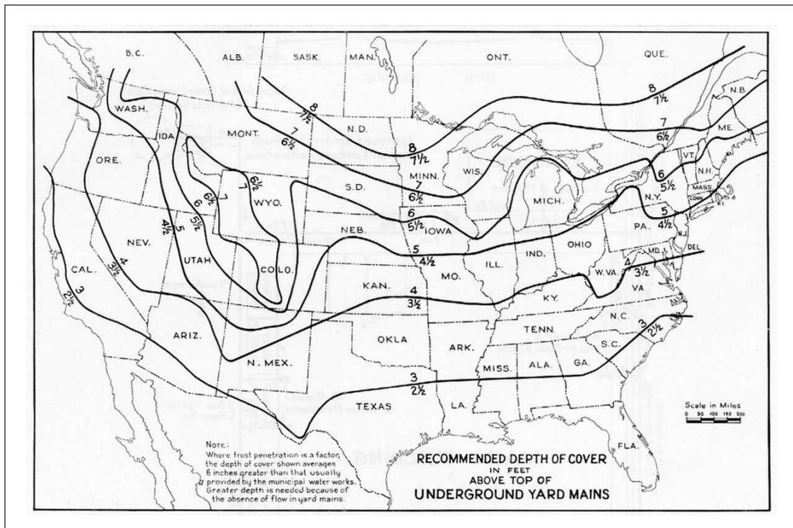
Fig. 37. Recommended depth of cover (ft) above underground mains (1 ft=0.3 m).
