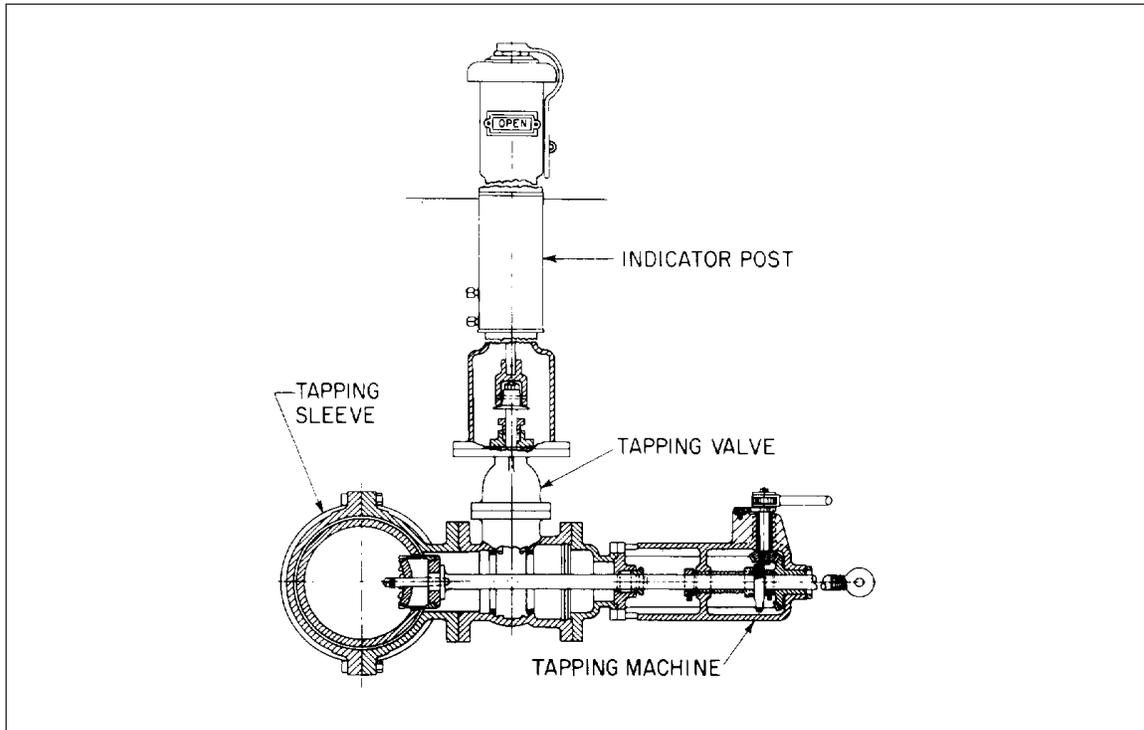
Fig. 39. Application of tapping machines to pipe under pressure (indicator post shown for reference only. Tapping is normally done without the indicator post attached.)
