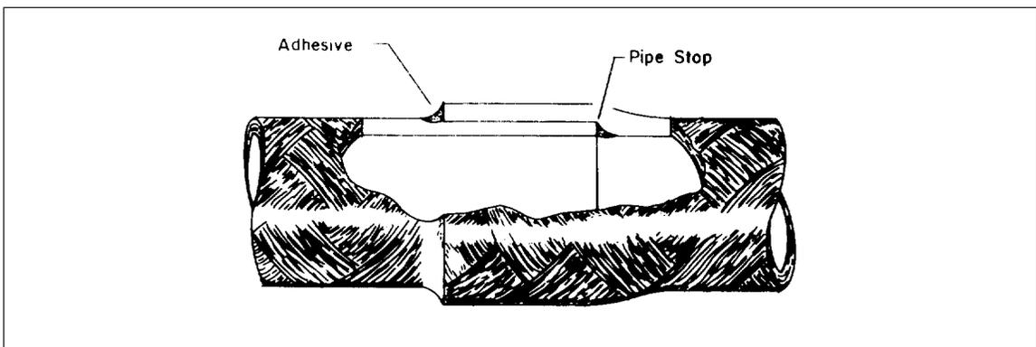
Fig. 26. Glass fiber-reinforced composite pipe joint formed by integral flanges and adhesive.
