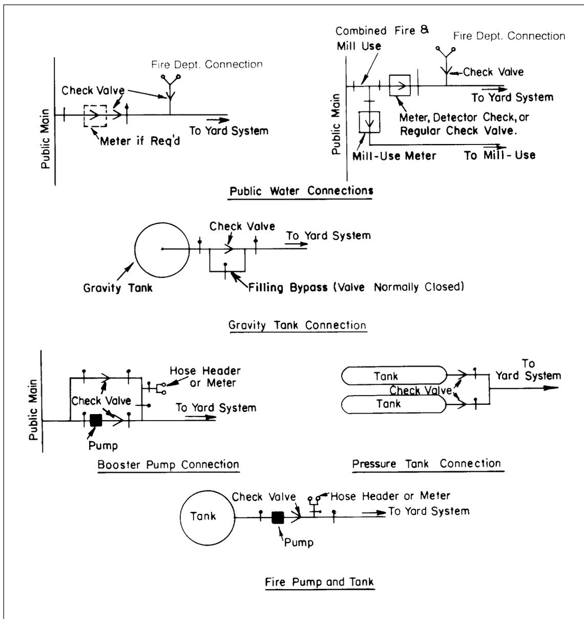
Fig. 28. Connections from water supplies.
