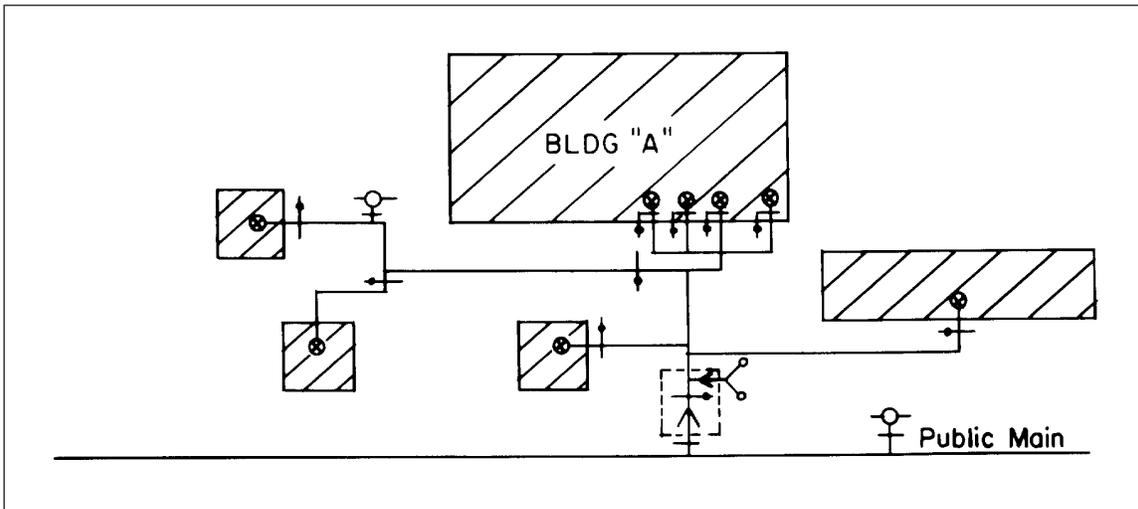
Fig. 32. System with manifolded riser arrangement.
