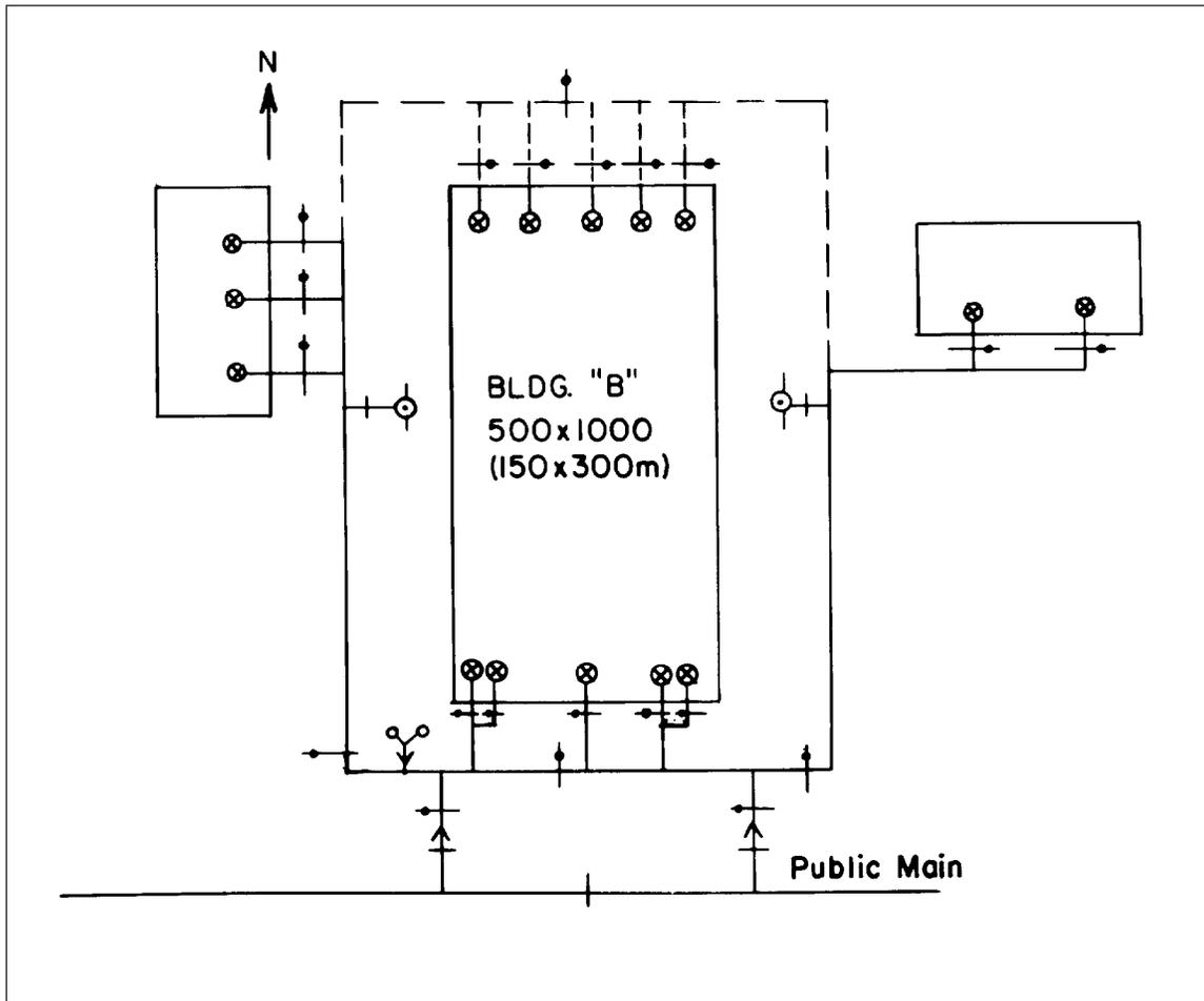
Fig. 34. System where completion of underground main loop avoids long runs of indoor feed mains.
