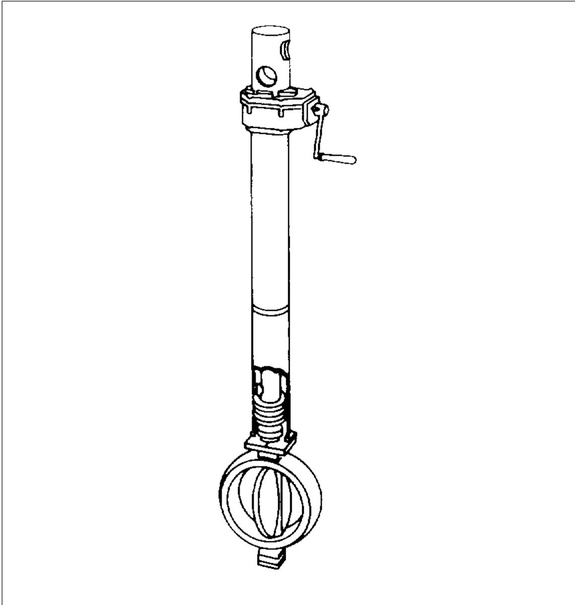
Fig. 11. Post indicator valve assembly.
