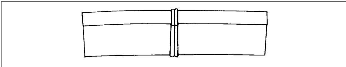
Fig. 23. Section of polyethylene pipe wall joined by butt fusion.
