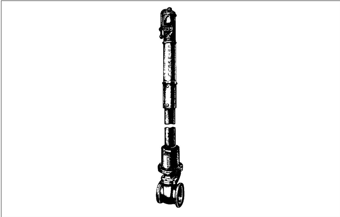
Fig. 12. Gate valve with indicator post.
