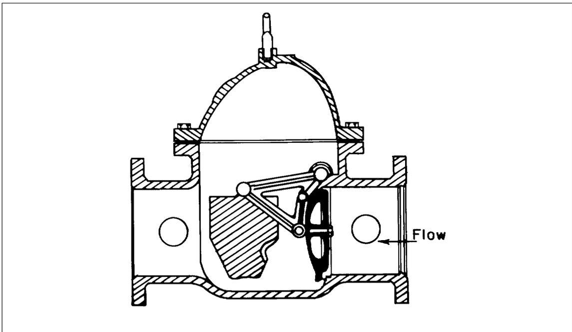
Fig. 3. Waterflow detector check valve, section view showing weighted clapper arrangement.
