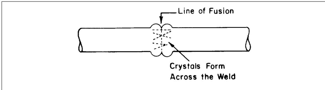
Fig. 22. Butt fusion joint.
