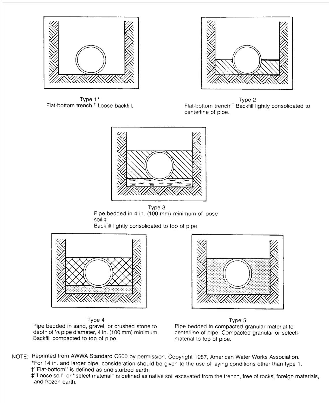
Fig. 35. Laying conditions for ductile-iron pipe.
