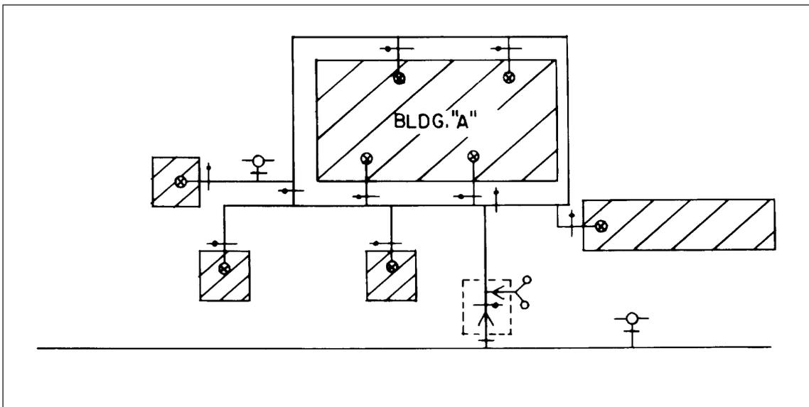
Fig. 33. System with looped main substituted for manifolded riser arrangement of Figure 32.
