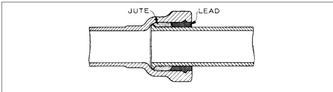
Fig. 20. Bell and spigot lead joint.
