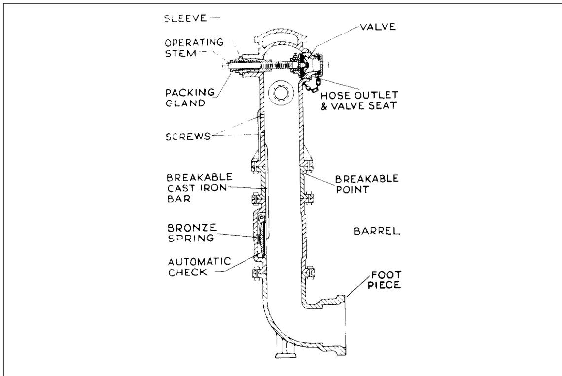
Fig. 17. Wet barrel hydrant.
