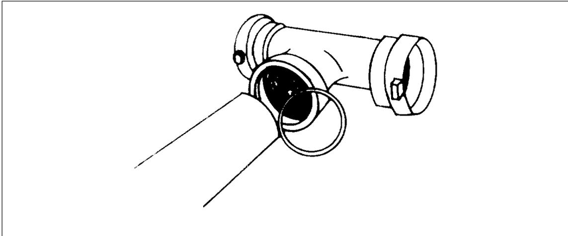
*Fig. 27. Glass fiber-reinforced composite pipe, cast iron fitting and transition gasket.*
