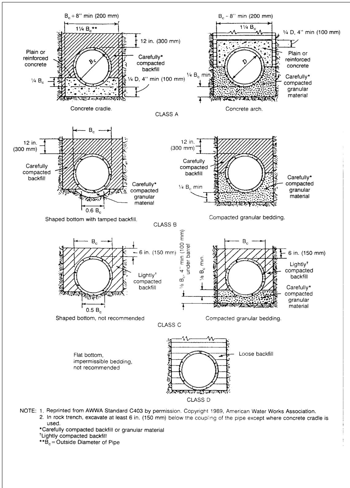
Fig. 36. Laying conditions for asbestos-cement pipe.
