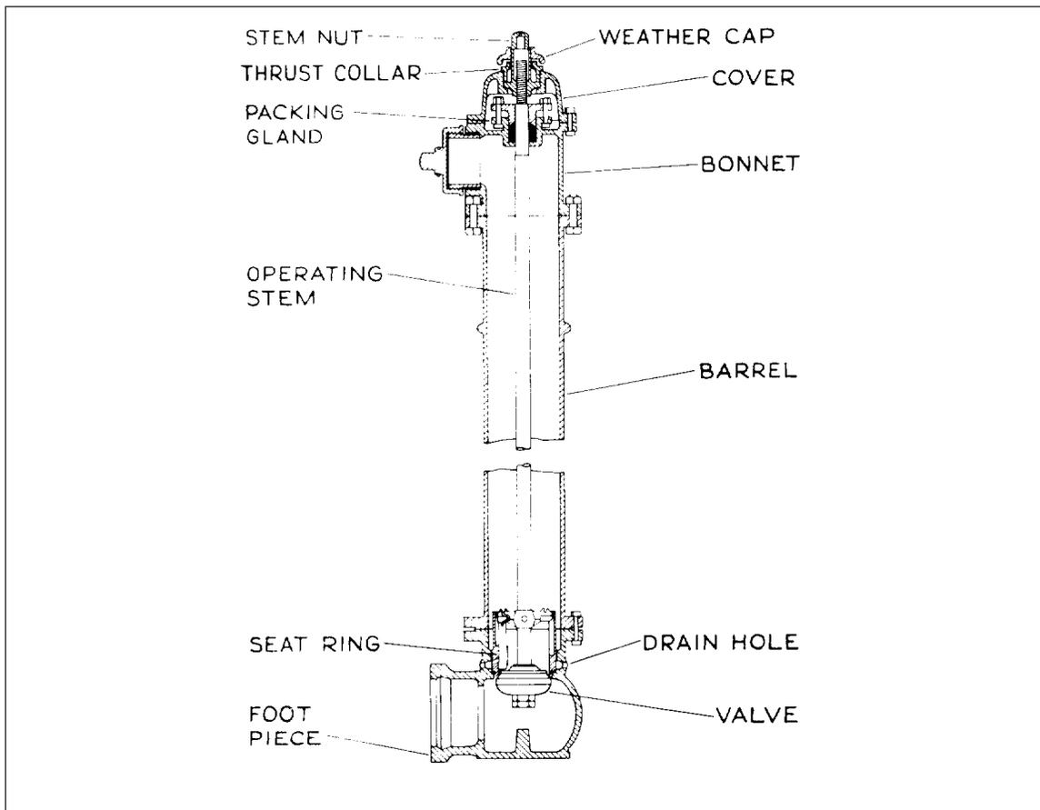
Fig. 16. Dry barrel hydrant.
