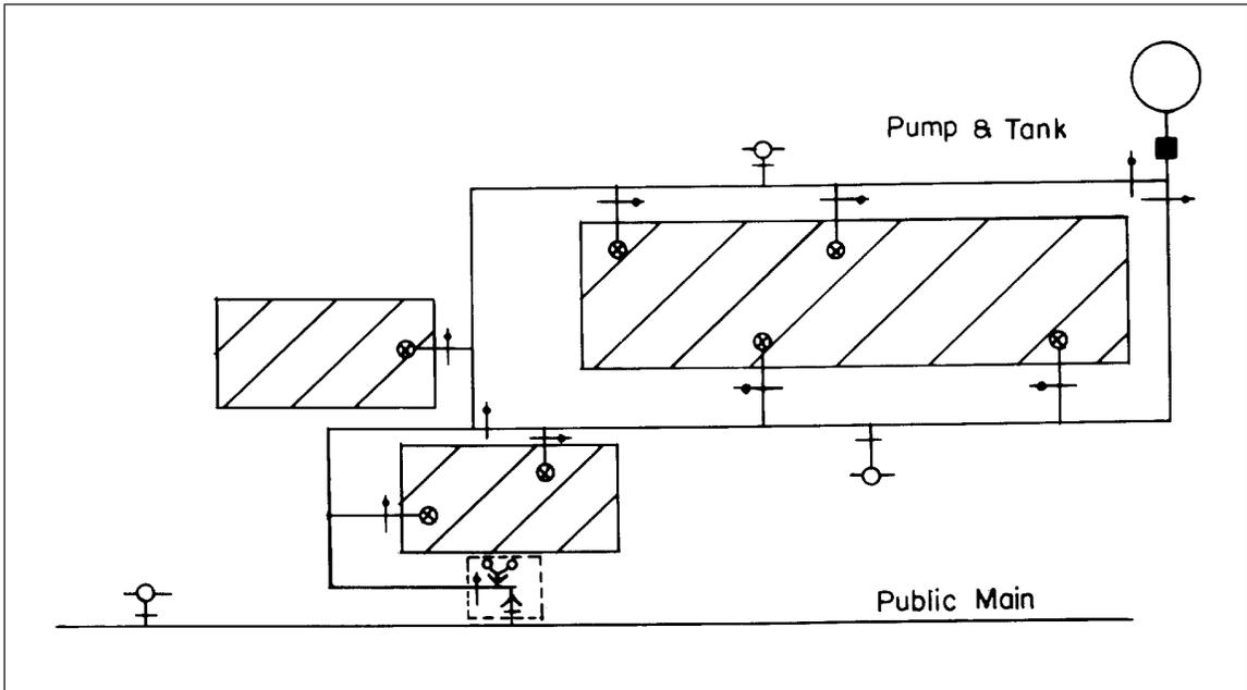
Fig. 31. Acceptable arrangement of multiple water sources.
