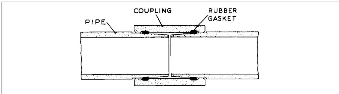
Fig. 21. Coupling for asbestos cement pipe.
