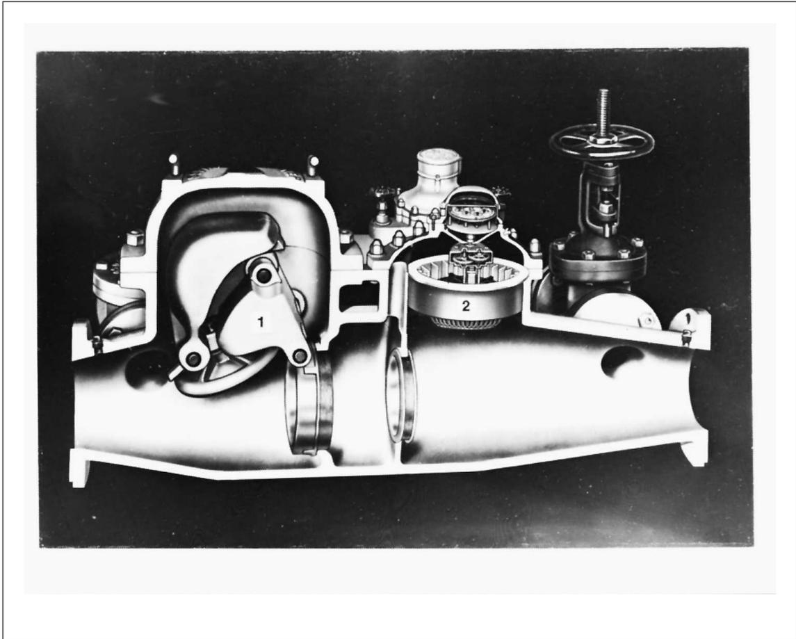
Fig. 2. Full registration fire service meter, section view showing weighted lever valve (1) and mainline torrent meter (2).
