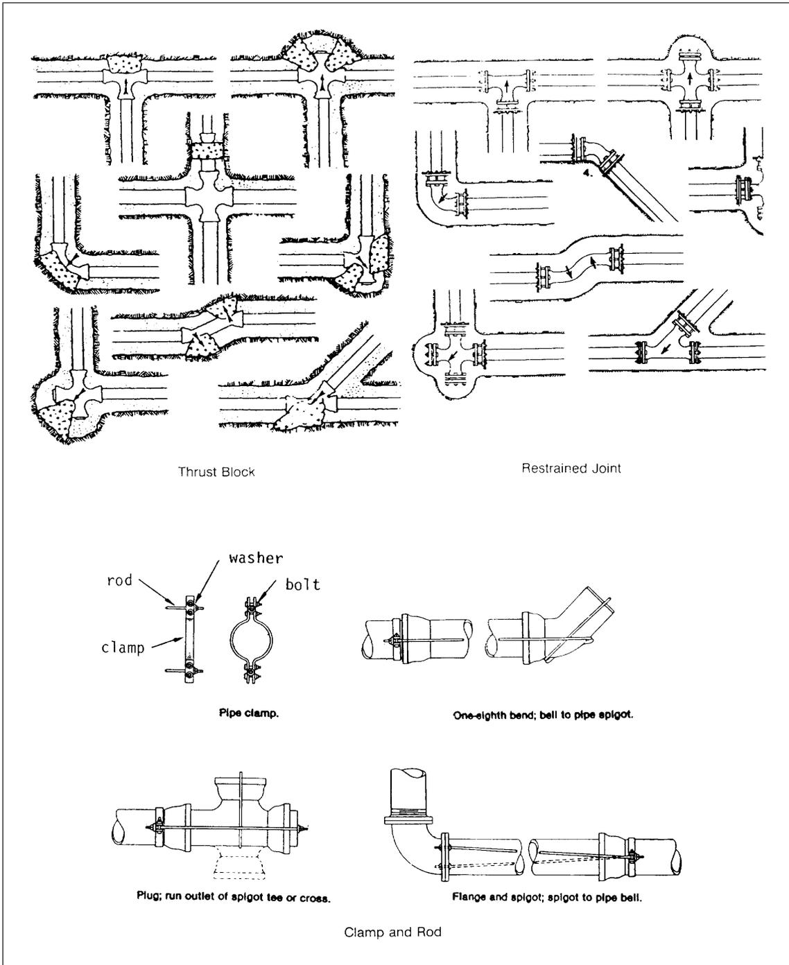
Fig. 38. Various methods of joint restraint.
