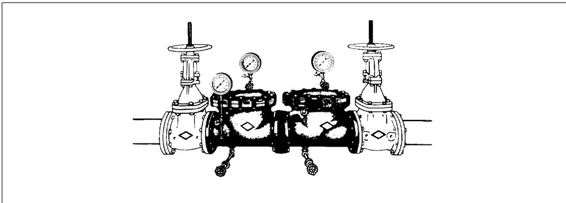
Fig. 8. Double check valve.
