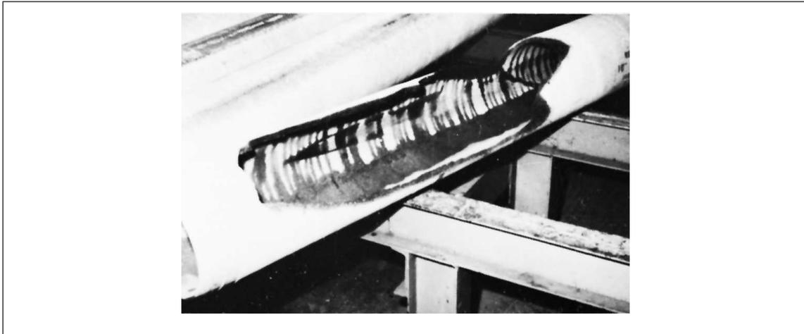
Fig. 41. High pressure hydro break.
