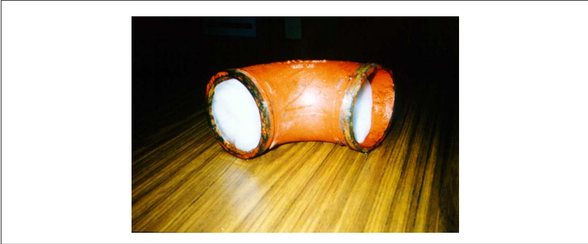
Fig. 3. Ice plug inside elbow
