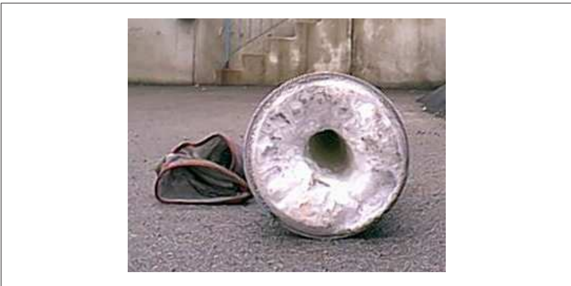
Fig. 4a. Ice plug on feedmain removed from the freezer.
