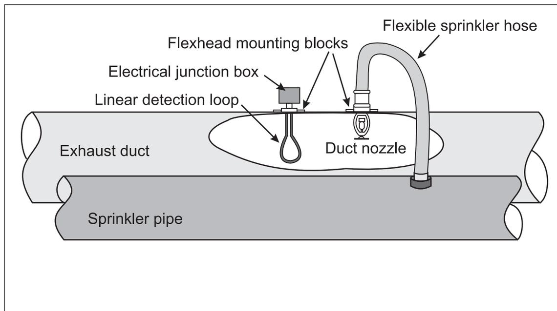
Fig. 2. Typical location of duct nozzle and linear heat detection wire in exhaust duct
