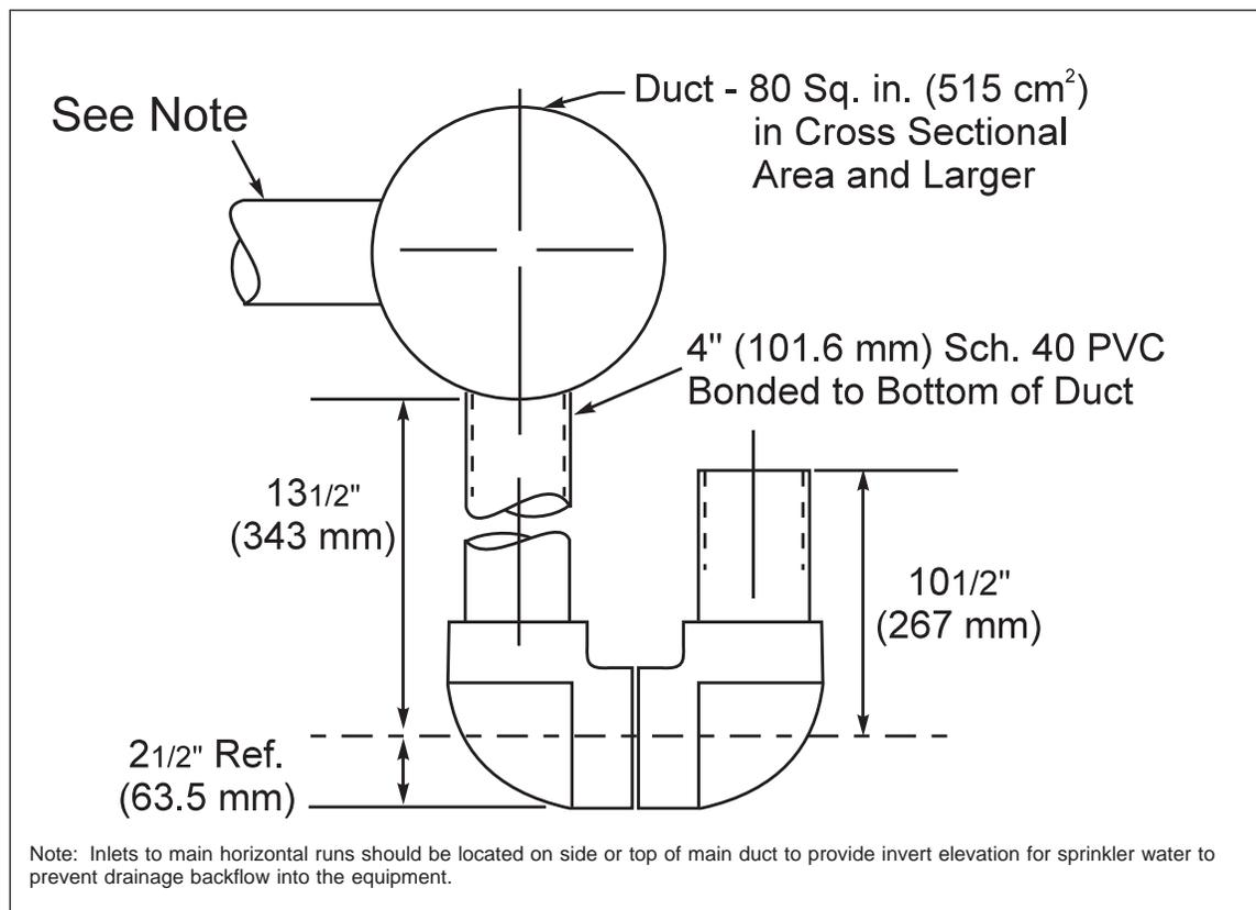
Fig. 1. Four in. (102 mm) drain
