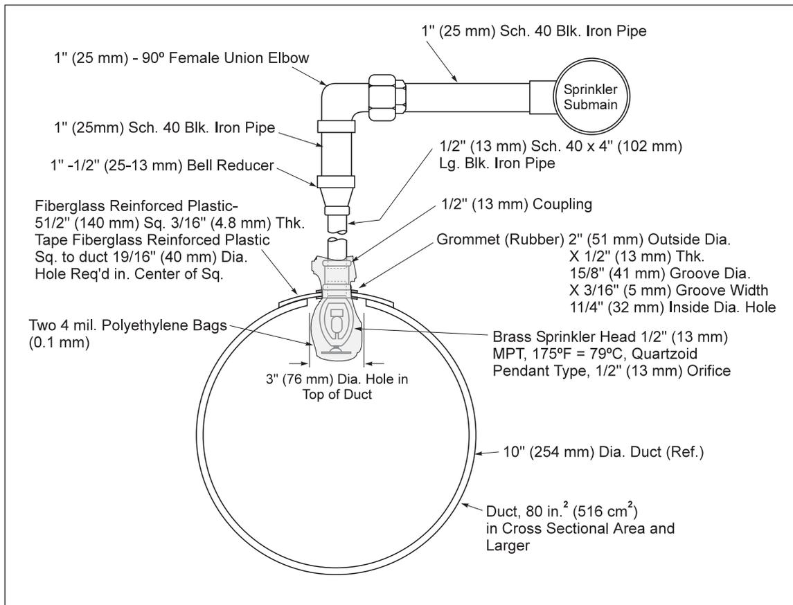
Fig. 5. Typical hard-piped sprinkler installation
