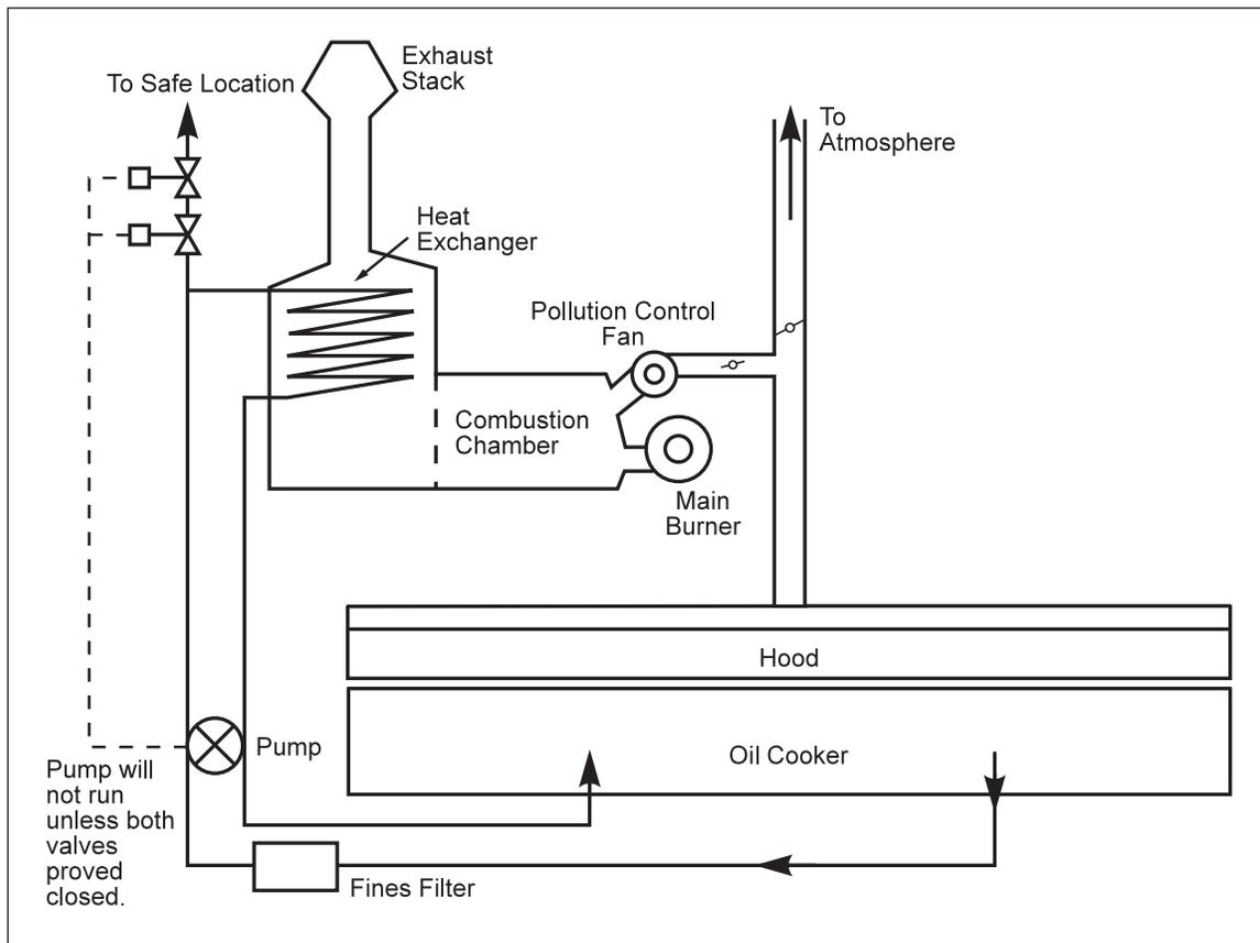
Fig. 2.4.2.8.E Cooking oil heat exchanger venting arrangement for detached heater/thermal oxidizer
