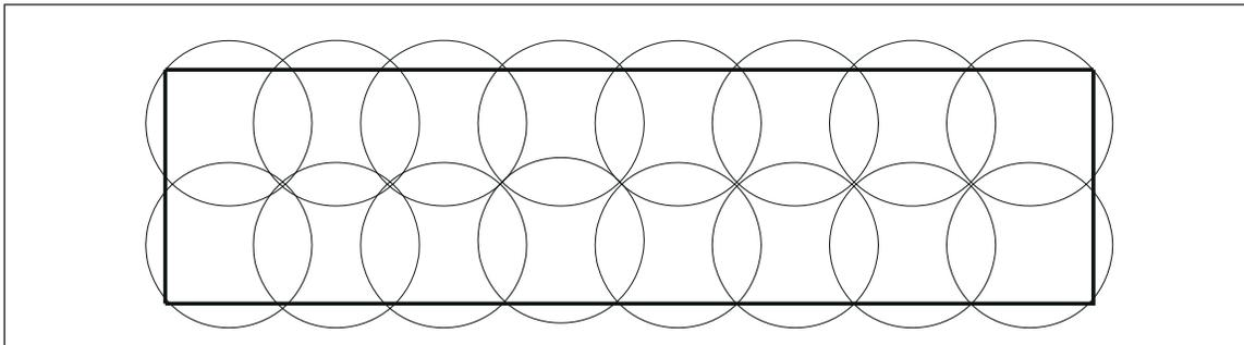
Fig. 2.4.2.4.B. Oil cooker nozzle spray coverage pattern
