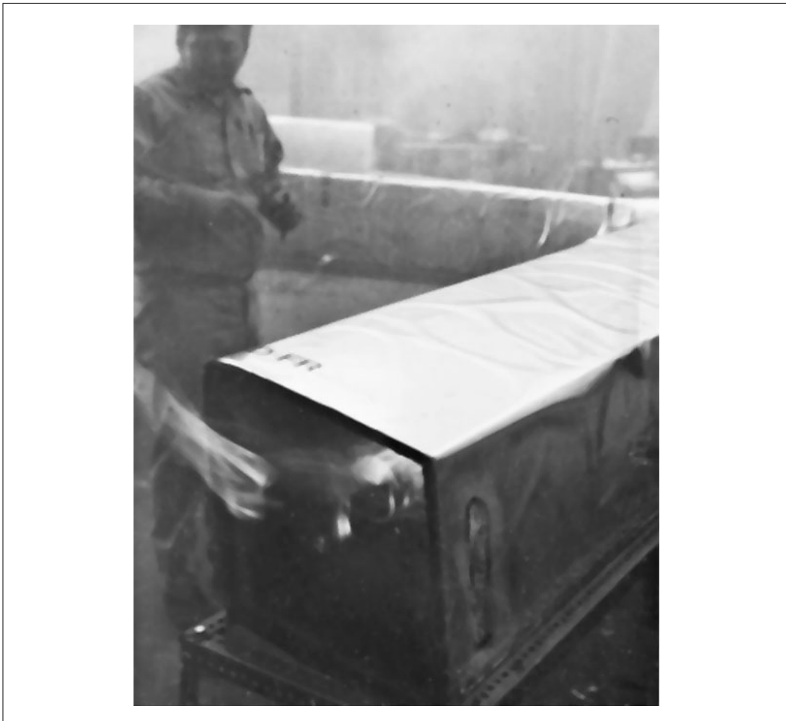
Fig. 3.4-2. A plastic duct that failed this test, despite a flame spread rating of 25 per the ASTM E-84 test
